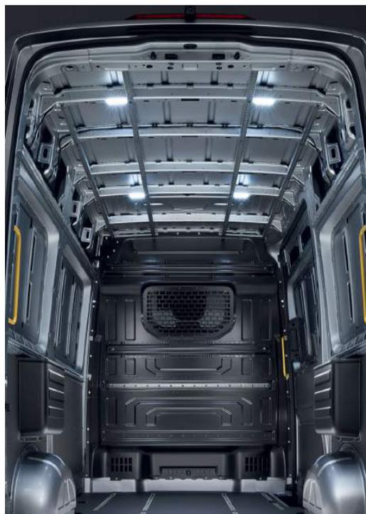
**06 Internal roof rack.\*** Enables easy transport of long objects. The two rails can be moved within the vehicle and adjusted to the length of the objects. They can also be removed when the roof rack is not needed.
