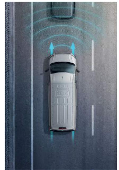
**Front Assist with City Emergency Braking System.**
