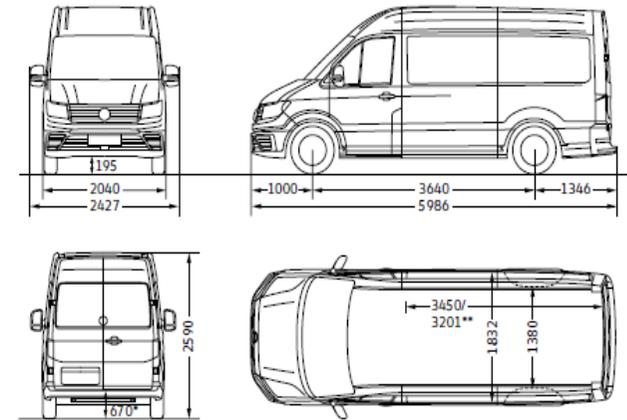
Illustration shown is CR35 medium wheelbase panel van with high roof.
