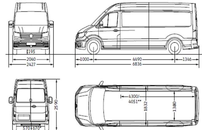
Illustration shown is CR35 long wheelbase panel van with high roof.
